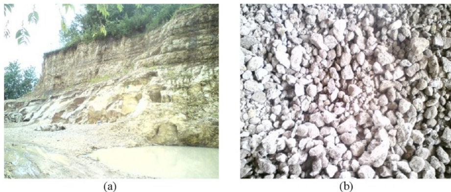
Figure 1: (a) Part of Pumice Breccia Deposit in the Semilir Formation, (b) Crushed Pumice Breccia
